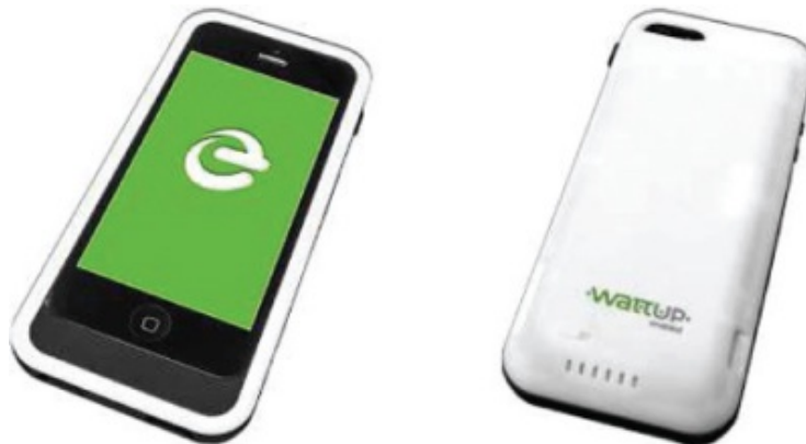
Figure 3: Front and Back of our Prototype Smart Phone Case with Embedded Energeous Receiver Technology
