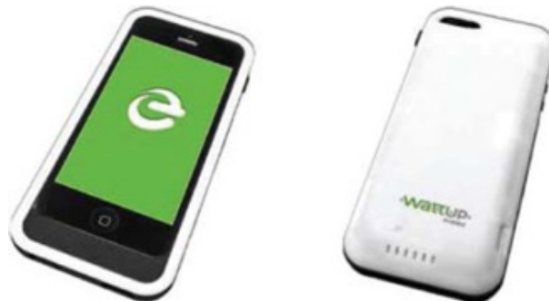
Figure 2: Front and Back of our Prototype Smart Phone Case with Embedded Energous Receiver Technology
